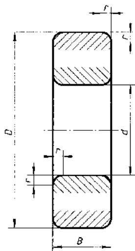
**Figure 1 — Radial bearing**
